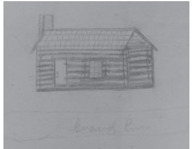
This sketch made by John S. Hooker in 1916 of Daniel Marsac's trading post which stood on the south side of Grand River facing the river. Its size was 16 ft by 26 ft. The logs were laid horizontally. Hooker also traded from this building.
