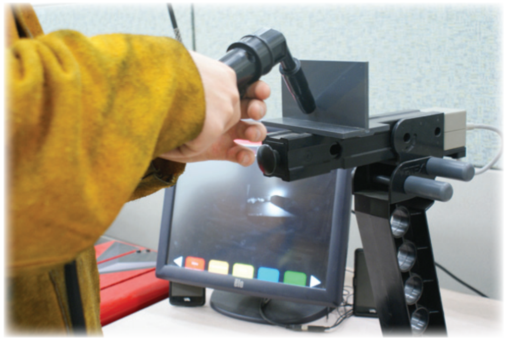
Practicing on the virtual reality welding machine. A small monitor allows those nearby to watch the student work.
