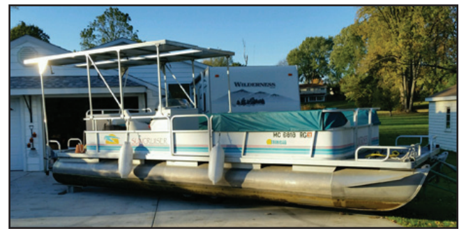
This pontoon boat named the Suncatcher has 1,300 watts of solar panels on its back. The conversion cost about $8,000. [photo courtesy Brad Kallio]
