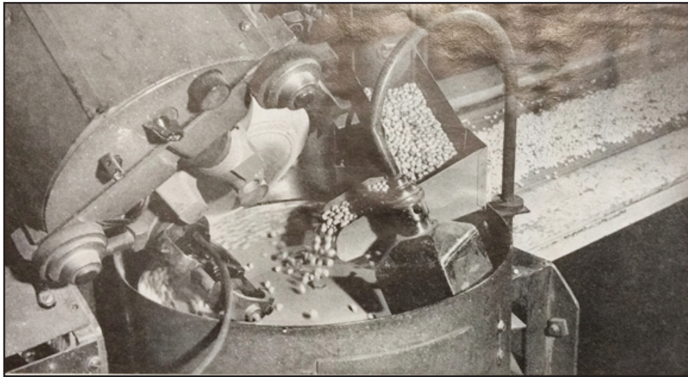
Runciman's electric eye bean sorter was the first in the world. [courtesy Lowell Area Historical Museum]
