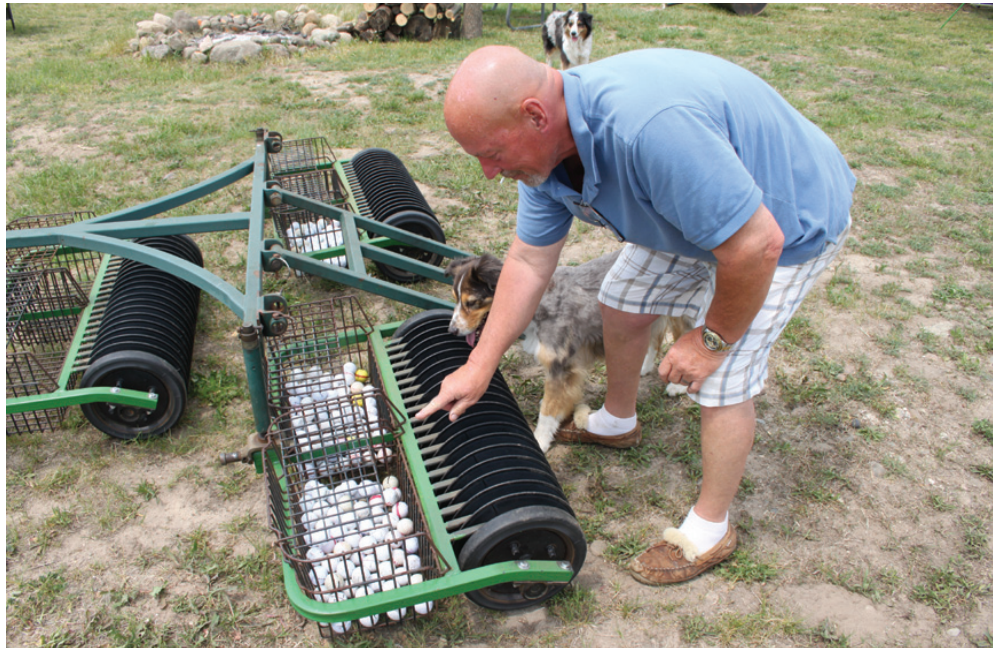
One of the main things Clausen picked up to help collect golf balls along the driving range was the ball picker, which he attaches to a four-wheeler and runs down each lane.
