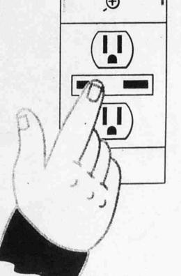
Ground fault circuit interrupters detect current leakages from appliances that you use everyday. When electric current leaks outside its path - through a damage wire, for example - GFCIs shut off the outlet. GFCIs can save you from severe shocks, burns, or electrocutions.
