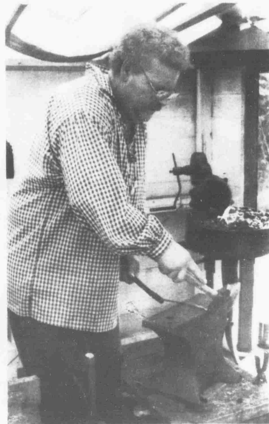
David Bradbury does a little blacksmith work like it was done back in the 1860's. Bradbury is making S-hooks which were used to suspend pots over the fire. Behind Bradbury, to his left, is a forge, used to fan the coals. This forgewas made in 1902. The anvil used to shape the steel was made in 1848 by William Foster.
