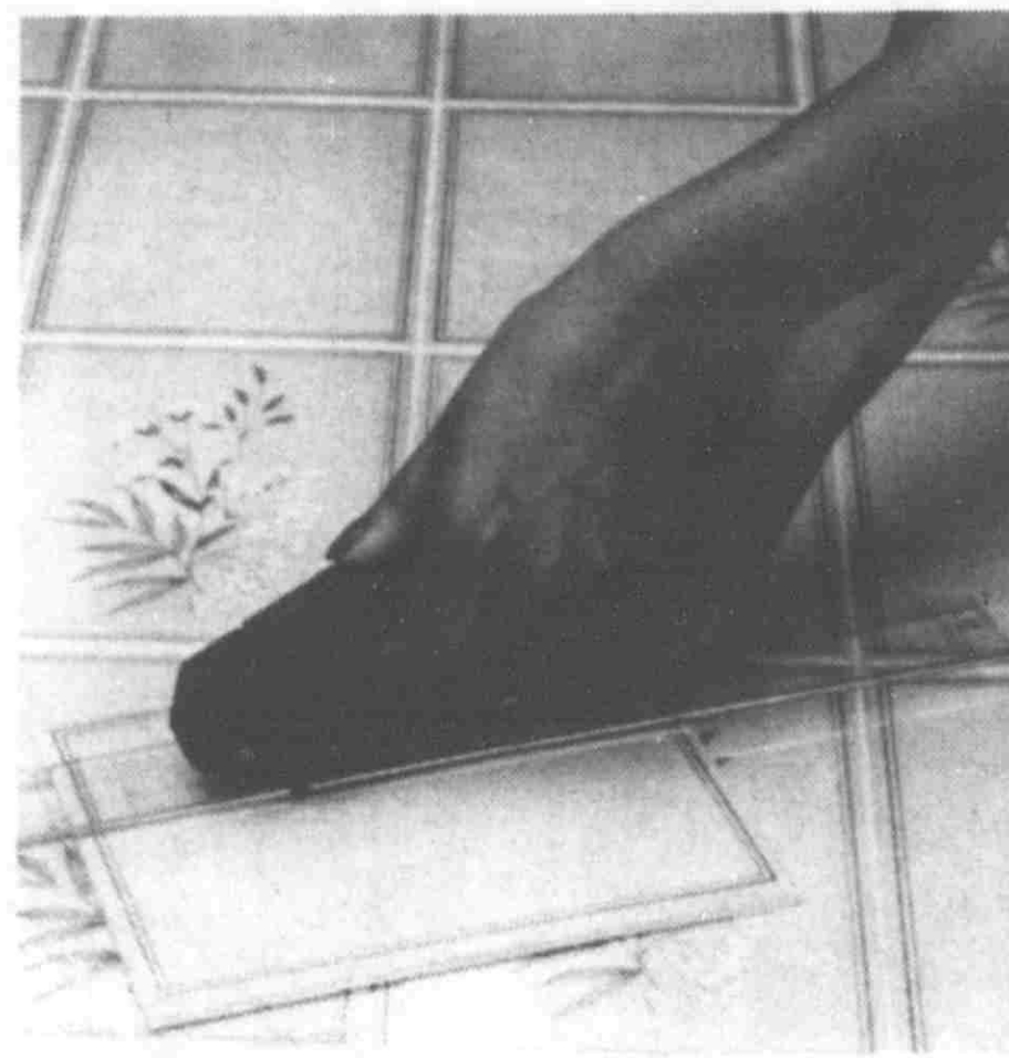
A tile cutter as illustrated, drastically reduces the time and myriad of tools needed for the simplest of tiling jobs.
