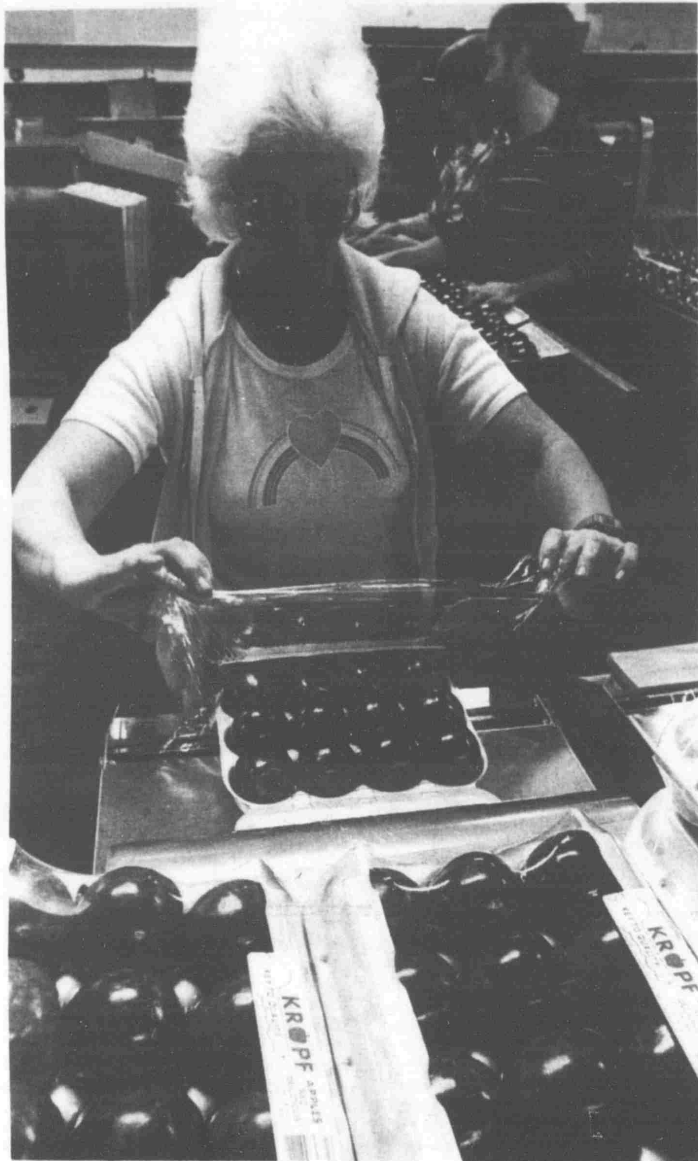
Glossy clear Goodyear Omnifilm puts the finishing touch on a special 12 Pack produce container designed to protect delicate fruit from being bruised. Apple grower and innovator Roger Kropf of Lowell, created the package to distribute the weight of stacked fruit without damage.
