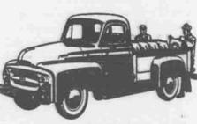
New Model R-110 pickup with 8-foot body. Other pickup models available with 61/2 and 9-foot bodies.
