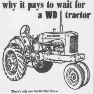
POWER-SHIFT rear wheels moved in or out by the engine TWO-CLUTCH control with foot-operated master clutch plus oil-cushioned hand clutch. Works like a second engine
