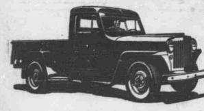
The truck that cuts having costs. Functional body with high-dearance fenders, wide-opening hood, comfantable cab. 118-in, wheelbase. 4700-5300 lbs. GVW.
