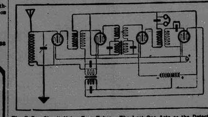
The Reflex Circuit Using Four Tubes. The Last One Acts as the Detector
