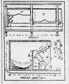
Details of Construction of Trap Nest.
