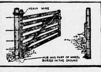
An Old Axle, With Parts of the Two Wheels Remaining Upon It Forms an Essential Part of This Easy-Working Farm Gate.
