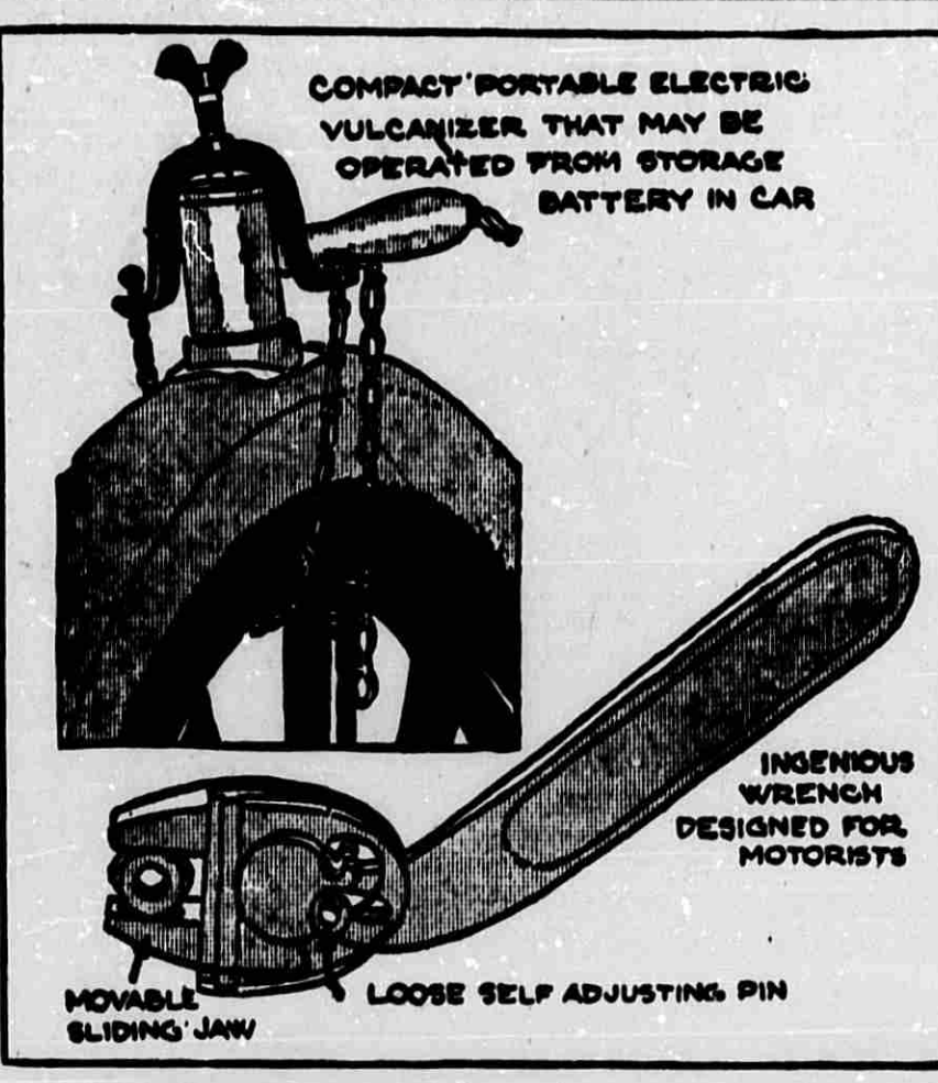
COMPACT PORTABLE ELECTRIC VULCANIZER THAT MAY BE OPERATED FROM STORAGE BATTERY IN CAR
