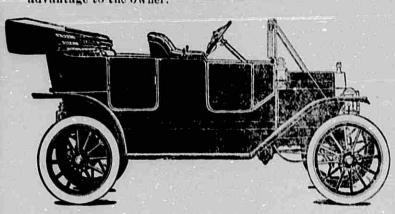
5-passenger, 4-cylinder, 20 horsepower car. Price, \$690, includes extension top, automatic brass windshield, speedometer, two 6-inch gas lamps, generator, three oil lamps, horn and tools. Fore-doors are detachable. f.o.b. Detroit.
