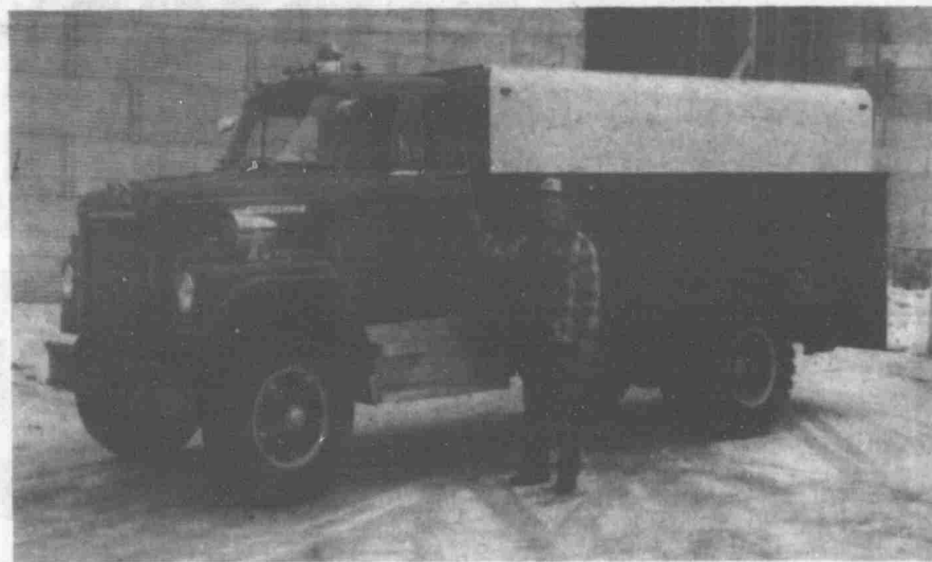
The latest addition to the Lowell Fire Department is this rescue equipment vehicle. The truck chassis was salvaged from an old Lowell pumper that was retired, and the equipment box was added by Allied Truck Equipment in Grand Rapids.
