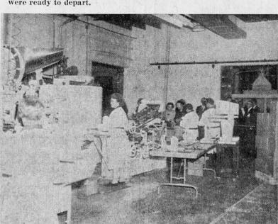
The visiting distributors are shown here inspecting the automatic liquid filling machine that fills, caps, weighs and labels the plastic bottles of the many products produced at the Ada plant.
